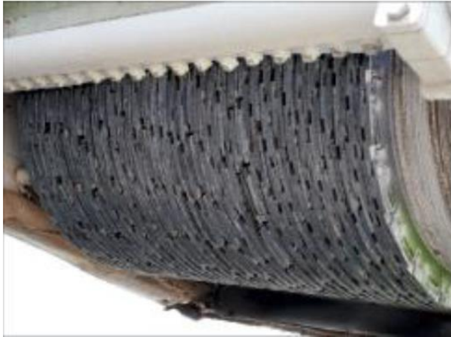
Figure A6-8. Diamond grinding of cement concrete
